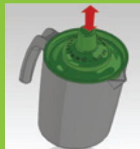
**6** Slide the inner chamber in and out of the jug 6 times, once a day.
